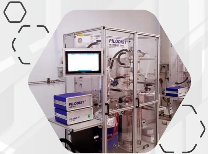
PETRODIST 200CC FULLY AUTOMATIC - Vacuum System to improve automatic pressure reduction, following the dynamic vacuum pressure procedure described in method ASTM D5236
